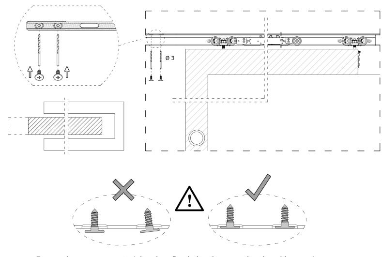
Ensure the screws are straight when fixed else the screw head could cause issues
