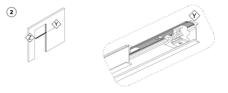
Remove the adjustable stops from the track at both ends.
